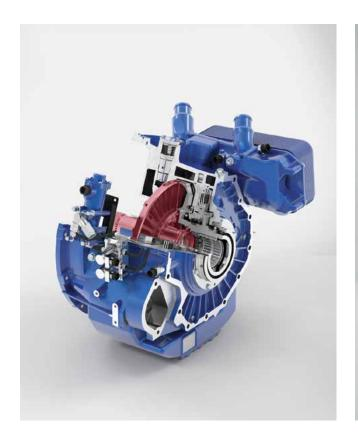
**Turbo retarder clutch.** The wear-free turbo retarder clutch<sup>2)</sup> offers maximum performance when moving off and enables manoeuvring for any duration. It also serves as a retarder, thus providing for additionally enhanced safety.
