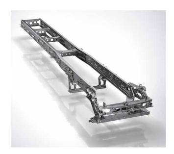
**Ideal framework.** The frame of the Arocs is available in two different widths and with longitudinal members of 7 mm, 8 mm and 9 mm in thickness. This allows the Arocs to be tailored ideally to the most diverse requirements in construction-site and road use.
