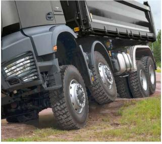
**Axle load compensation.** The axle load compensation <sup>11</sup> between the front axles prevents damage due to overloading and reduces wear on the axle suspension, steering and tyres. Other benefits are easy handling, high ride comfort and improved distribution of braking forces.
