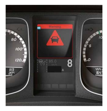
Active Brake Assist. Within the system's limits, Active Brake Assist can detect obstacles driving ahead of the vehicle, warn the driver of dangers identified and, if necessary, carry out a full brake application to mitigate the severity of a possible accident and its consequences.
